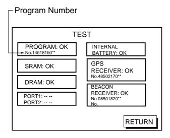
Figure 11-21 Memory, I/O test results
